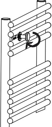
A technical line drawing showing the towel rack base being tightened onto a frame. A curved arrow indicates the direction of rotation for the screw, showing it being tightened.                                                             |
